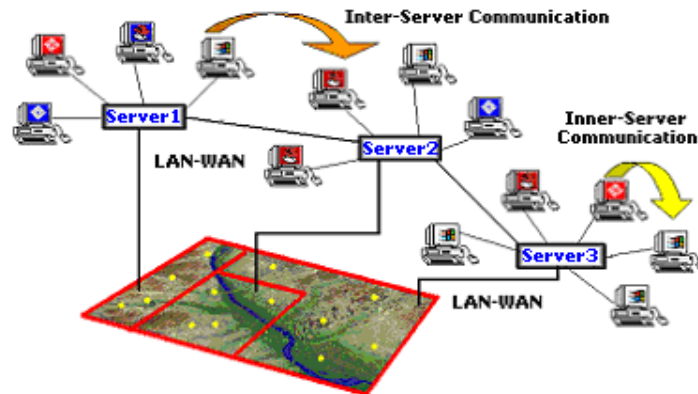
Figure 30 - A multi-server architecture for a basic DVE
