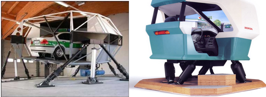
Figure 15 - 6-DOF Spider System for Vehicle Simulator (from FCS Simulator Systems) and Honda Car Driving Simulator
