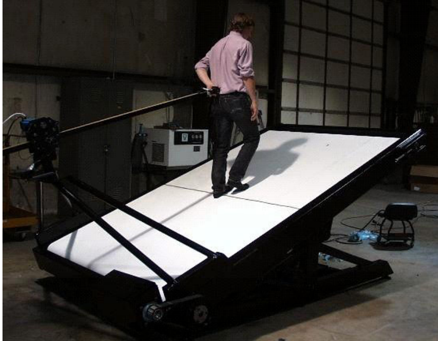
Figure 23 - Locomotion System with Vestibular feedback developed by Prof. Hollerback
