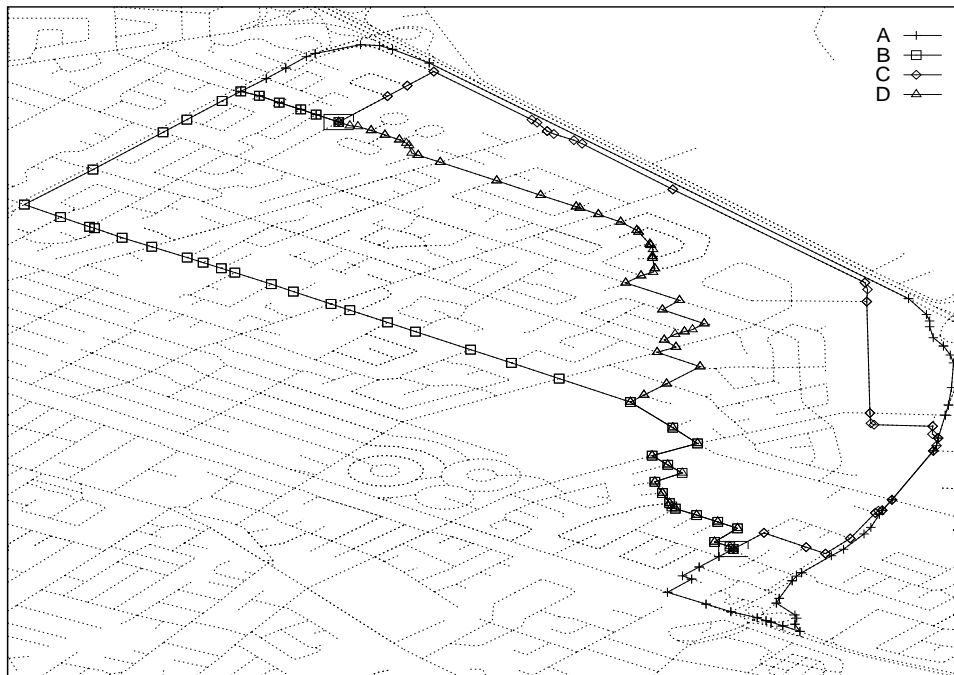
Figure 5: Sample task for the subjects. The starting point is the box at the upper left and the ending point is the box at the lower right. A is the route with fewest turns, B is the fastest route, C is the route with fewest intersections, and D is the shortest route.
