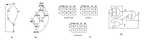
Figure 1: (a) STG, (b) SG, (c) next-state functions, (d) complex-gate implementation.
