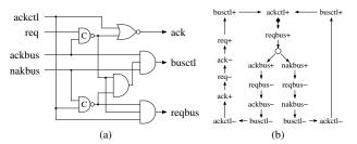
Fig. 8. Circuit and mined specification for alloc-outbound.
