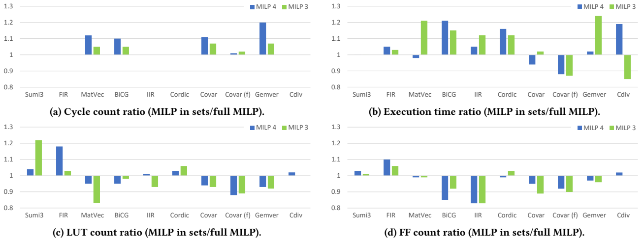
Figure 9: Comparison of solutions obtained by applying the MILP on individual CFDFC sets with the optimal MILP solutions (i.e., solutions obtained by employing the MILP on the entire circuits).
