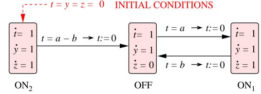
Safety requirement: heater on < 40% of the first 60 seconds  $\rightarrow$  proved using polynomial invariants
